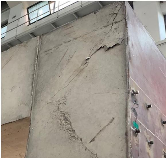
Failure mode of No.6 L-CM-JS-I
