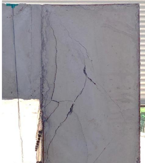
Failure mode of No.2 L-OM-JS-I
